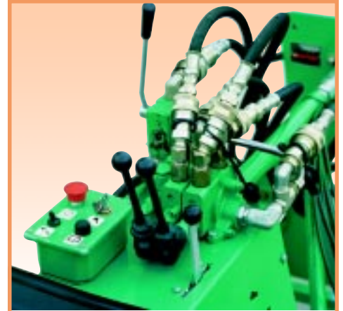
Alignment corrections and direction changes are easily made with joystick controls that maneuver both ends of the screed separately.
