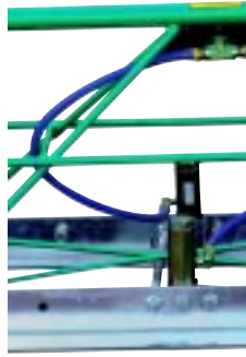
Naval bronze air vibrators are rust resistant and deliver high frequency vibrations.
